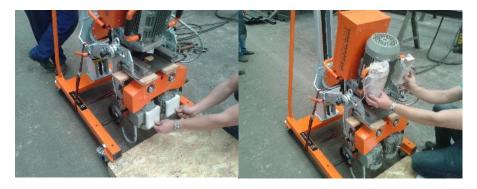
$6\slash$  Lay the UZ50 on the palette according the picture.
