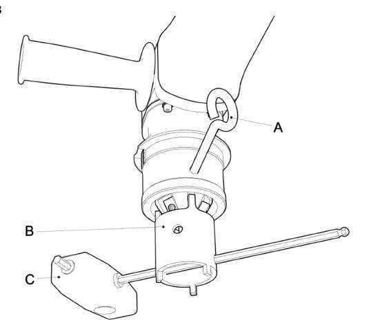
Always, when the milling head is replaced, treat the head thread and the screw with copper-containing grease (copper paste). This paste prevents the thread of the milling head from being jamed / sealed and facilitates future loosening.
